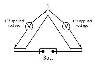
2. Connect the 1-4-9 circuit as shown. 4&9 are connected to the battery terminal. 1 is flashed with the other battery terminal. A strong deflection will occur across leads 2&7 and across leads 3&6. Little or no deflection will be seen across leads 2&5 and 3&8. Leads 5,6,7, and 8 can now be labeled.
